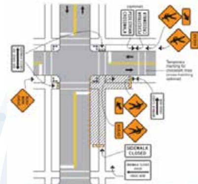
Crosswalk Closures and Pedestrian Detours
